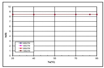
Figure 4: Encased Converter (0.9" heatsink) max. output current derating vs. ambient air temperature for airflow rates of 100 LFM through 400 LFM. Air flows across the converter from input to output (nominal input voltage).
