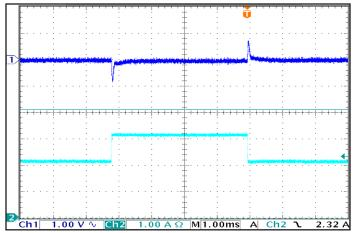
Figure 5: Output voltage response to step-change in load current (50%-75%-50% of lout(max);  $dI/dt = 0.1 A/\mu s$ ). Load cap:  $1 \mu F$  ceramic capacitor. Ch 1: Vout, Ch 2: lout (IA/div.)
