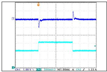
Figure 5: Output voltage response to step-change in load current (50%-75%-50% of Iout(max);  $dI/dt = 0.1 A/\mu s$ ). Load cap:  $1 \mu F$  ceramic capacitor. Ch 1: Vout, Ch 2: Iout(0.5A/div).
