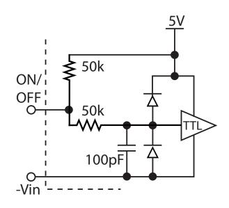
Figure B: Internal ON/OFF pin circuitry
