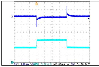
Figure 5: Output voltage response to step-change in load current (50%-75%-50% of Iout(max); dI/dt = 0.1 A/µs). Load cap: 1 µF ceramic and 15 µF tantalum capacitors. Ch 1: Vout, Ch 2: Iout (5A/div.)
