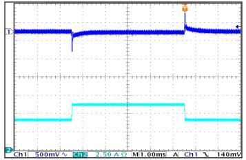
Figure 5: Output voltage response to step-change in load current (50%-75%-50% of lout(max); dI/dt = 0.1 A/µs). Load cap: 1 µF ceramic and 15 µF tantalum capacitors. Ch 1: Vout, Ch 2: lout (2.5A/div.)
