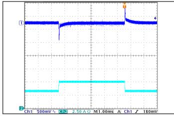
Figure 5: Output voltage response to step-change in load current (50%-75%-50% of lout(max); dI/dt = 0.1 A/µs). Load cap: 1 µF ceramic and 15 µF tantalum capacitors. Ch 1: Vout, Ch 2: lout (2.5A/div).
